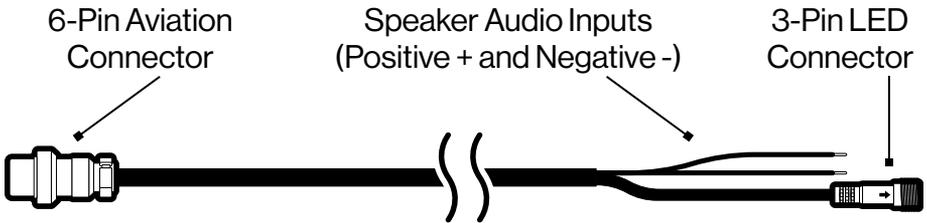
“Round C” 6-Pin Pass-Through LED and Speaker Aviation Cable
