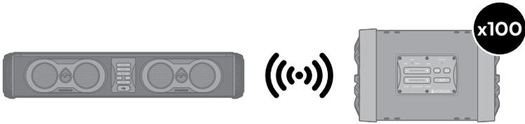
The ECOXGEAR SoundExtreme speaker is designed to be paired with one or more SoundExtreme speakers and Extreme Subs. You can build a broadcast system by initiating EcoCast Transmitting Mode in one SoundExtreme speaker and broadcasting your music to one or more Extreme Subs and SoundExtreme speakers in EcoCast Receiving Mode.
