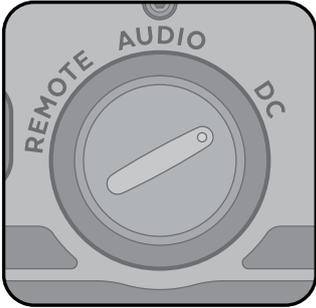
If you don't have an external control signal connection, you can turn the Auto-Turn-On switch to the **Audio** position to put the Extreme Sub into standby mode, reducing power consumption, when not in use.
