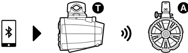
If there is an EcoCast-enabled speaker in EcoCast Transmitting Mode nearby, you can set your Amplified Tower Speaker (**Speaker A**) to EcoCast Receiving Mode and play audio streams from the EcoCast Transmitting speaker (**Speaker T**):
