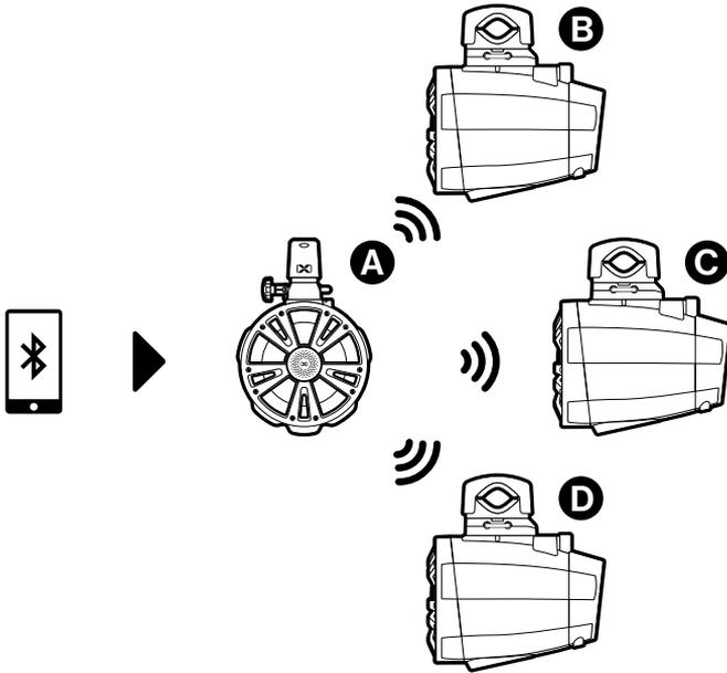
1. Turn on the additional EcoCast-enabled speakers (**Speaker C** and **Speaker D**) and press the Mode Button to cycle through to and initiate EcoCast Receiving Mode. The Mode LED Status Indicator will flash Green, and the speaker will announce, "EcoCast receiving."
