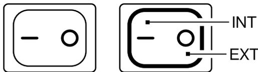
The Amplified Speaker has a built-in FM Antenna. It also includes an FM Dipole Antenna Jack for an optional external antenna connection and improved reception (dipole antenna sold separately). Next to the Power Mode Switch is the FM Antenna Switch (Blue Switch).
