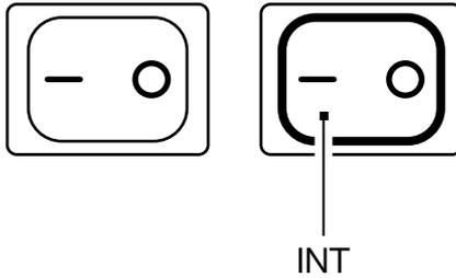
The first time you listen to FM Radio on your ExtremeTower Speakers, check the FM ANT Switch position to make sure it is in the correct position. If you use the Internal Antenna, the switch should be in the INT position.
