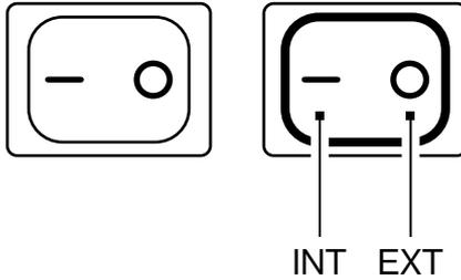
3. Open the Back Cover (refer to **Install the Rechargeable Battery Pack to the Amplified Speaker** for details), move the (Blue) FM ANT Switch to the EXT position.
