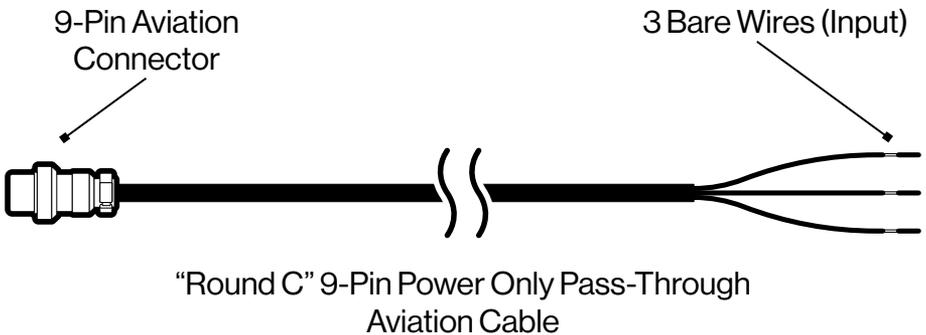
1. Aviation Cable Set — For easy running and fishing wires through a crossbar. The Aviation Cable connection between a 12V power supply and each Amplified ExtremeTower Speaker uses the following cable:
