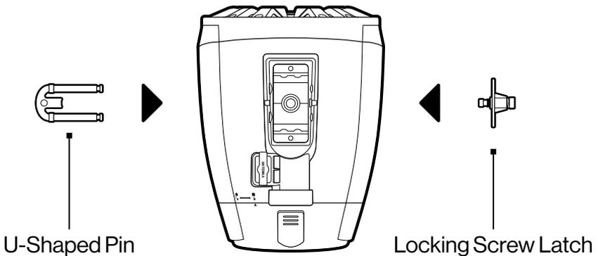
7. Insert the U-Shaped Pin into the two holes on the side of the Base-Mount. Insert the pins into the holes on the left side of the Mount when viewing from the rear of the speaker.
