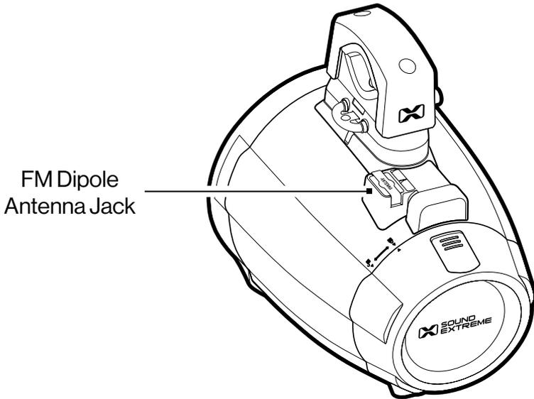
The Amplified Speaker has a built-in FM Antenna. It also includes an FM Dipole Antenna Jack for an optional external antenna connection and improved reception (dipole antenna sold separately). If you prefer to use an external FM antenna, follow these steps:
