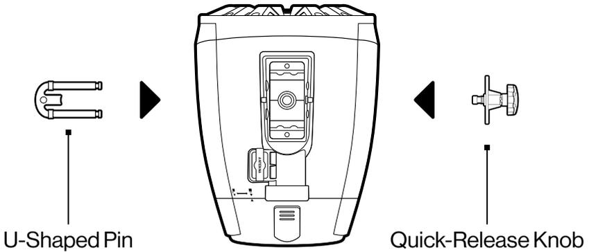
4. Insert the U-Shaped Pin into the two holes on the side of the Base-Mount. Insert the pins into the holes on the left side of the Mount when viewing from the rear of the speaker.
