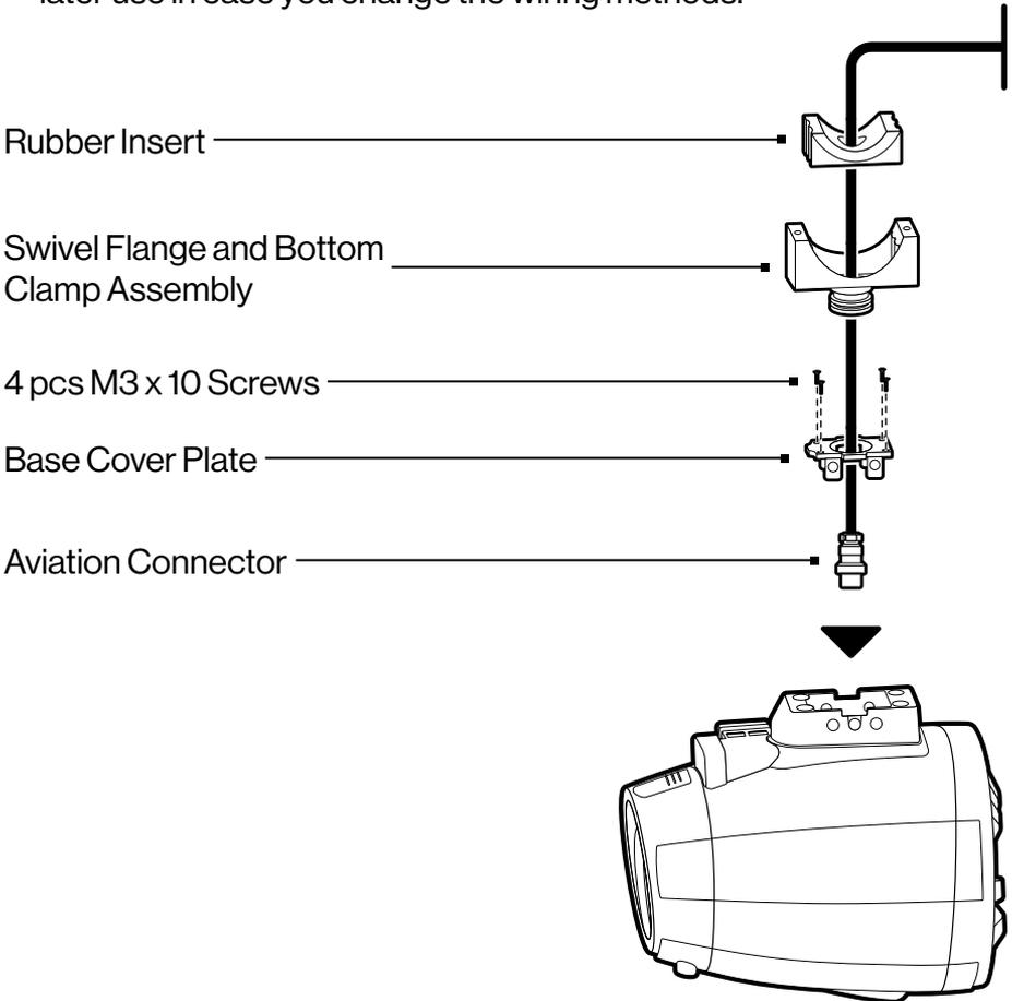
2. Put the appropriate Lower Rubber Insert onto the Swivel Flange and Bottom Clamp Assembly.
