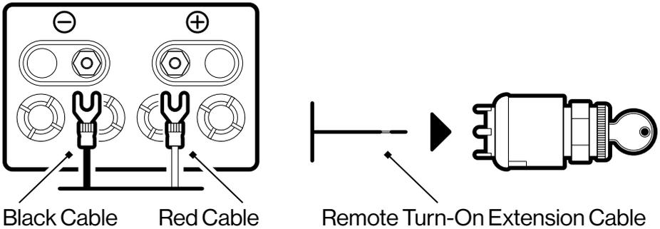
1. Once you complete one of the Installation Procedures, you can connect the 3 wires (+12V, GND, and Remote Turn-On) on the Power Cables (or Extension Cables, if needed) to the vehicle's battery and ignition signal terminal.
