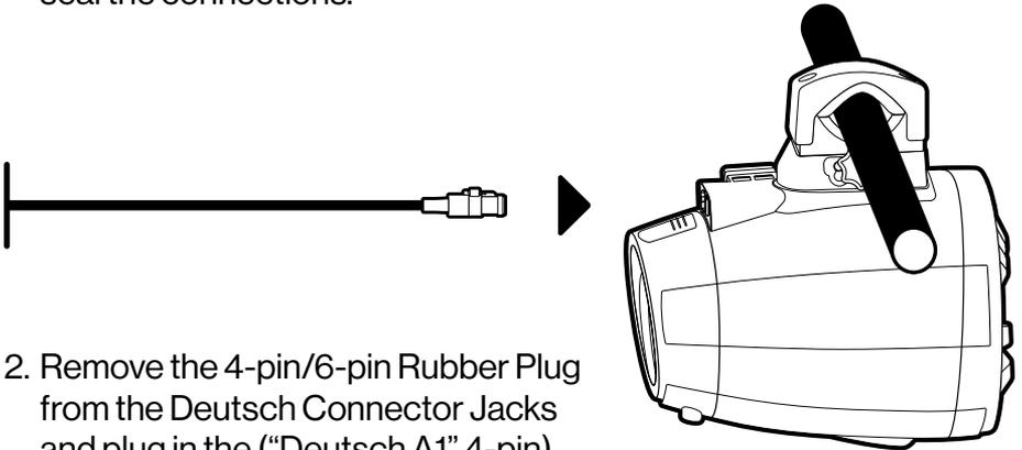
2. Remove the 4-pin/6-pin Rubber Plug from the Deutsch Connector Jacks and plug in the ("Deutsch A1" 4-pin) Deutsch Power Cable's connector into the 4-pin Deutsch Connector Jack on each speaker.
