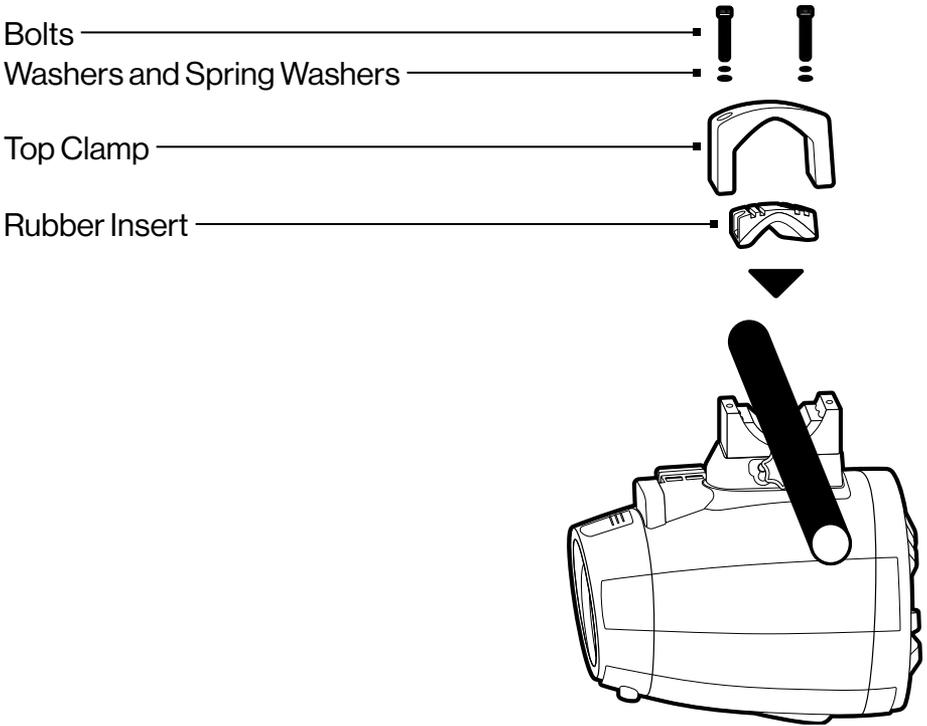
6. Put the Upper Rubber Insert on the Top Clamp. Align the rubber groove with the bulge of the Top Clamp and press down to assemble the Clamp and Rubber Insert.
