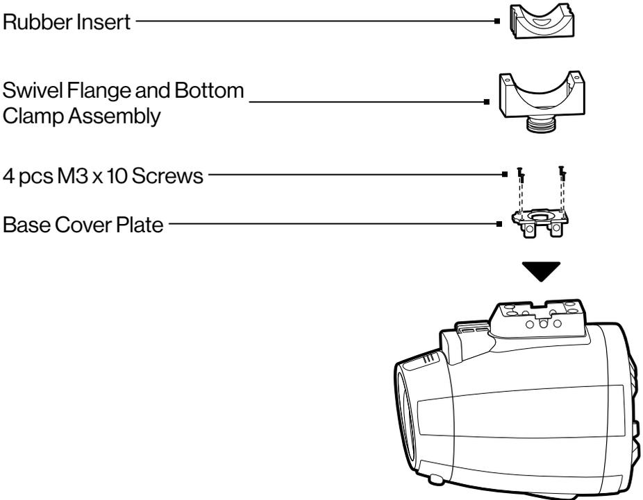
1. Put the appropriate Lower Rubber Insert onto the Swivel Flange and Bottom Clamp Assembly.
