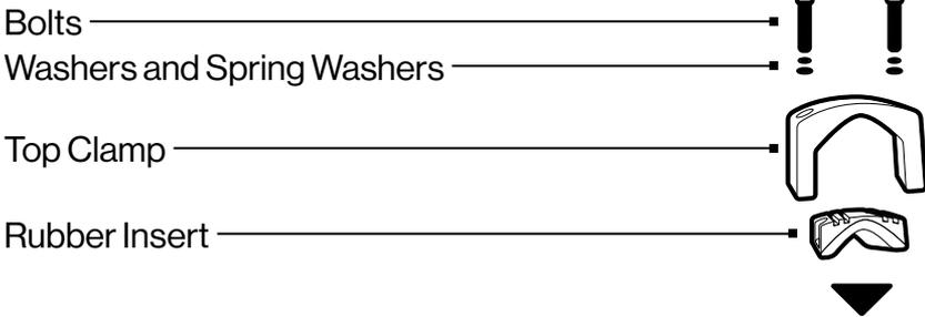
9. Put the Upper Rubber Insert on the Top Clamp. Align the rubber groove with the bulge of the Top Clamp and press down to assemble the Clamp and Rubber Insert.
