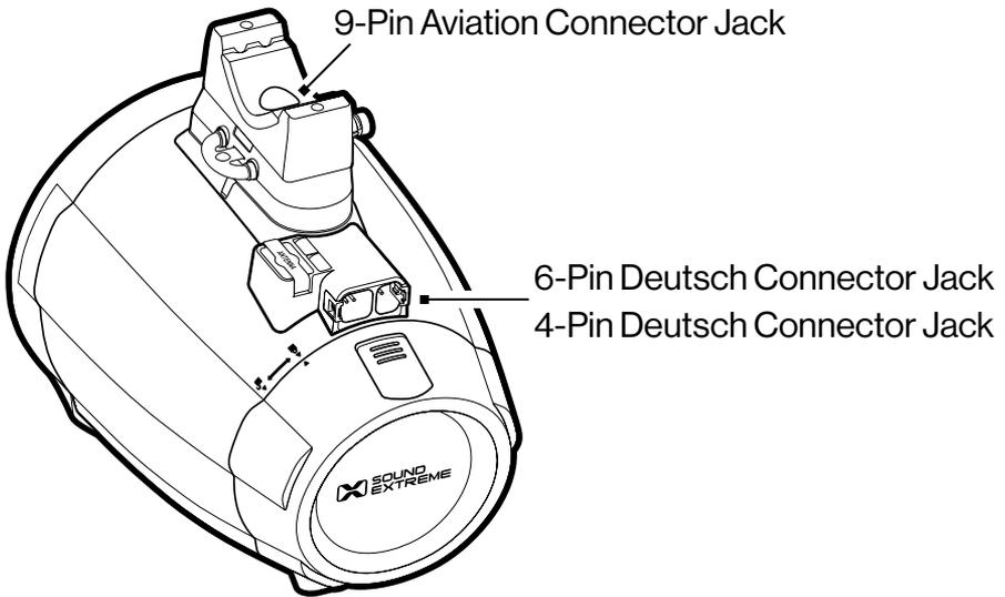
1. A round **Aviation Connector Jack** is inside the speaker Base-Mount, which allows the cable to pass through the Bottom Mount Clamp and go into a hole in the crossbar at the location where the speaker is mounted. These Amplified ExtremeTower Speakers have a 9-pin, round connector jack.
